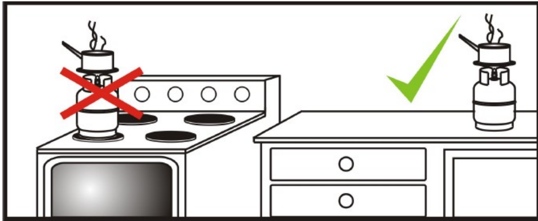
Figure D.1 — Correct and incorrect placement of cylinders
